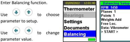
Set **RPM** of the machine at which balancing will be conducted.
