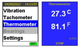
Device displays measurement result in °C and °F
