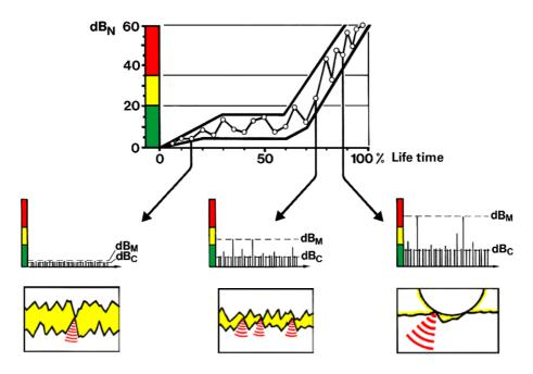
An increase in the carpet dBc value can be caused not only by deterioration in the condition of the lubricant, but also by other causes, such as misalignment of the shafts in the coupling of the drive. It is quite easy to distinguish between these phenomena: if the shafts are skewed, the same pattern will be observed for the bearings on both sides of the coupling.
