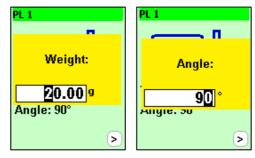
Run the machine and take measure vibration levels at all four points when trial weight is attached at the Plane #1.
