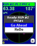
Stop the machine. Choose to keep or remove the trial weight at the Plane #2
